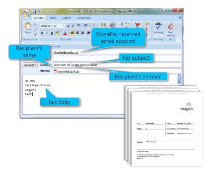
It is also possible to send a fax specifying destination number straight into "To:" field. For example: 123456789@digitalfax.mycompany.com (this option must be enabled by your email administrator).
