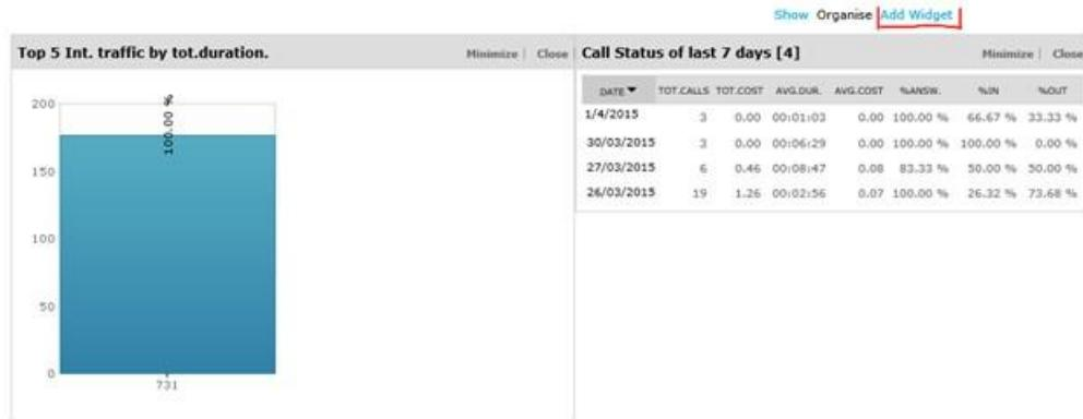
Each widget can be removed by clicking on relevant “Close” option, or it can be minimized (reduce to a single line) by clicking on “Minimize” button.
