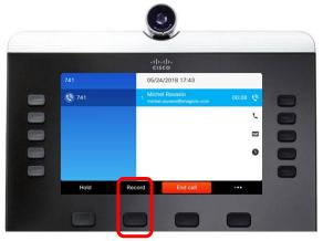
To stop recording, just hit the "Stop rec" button or hang up.
