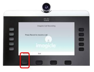
Within the call recording phone service screen, you can trigger the recording of current call. If Live Keep method is in use, the whole conversation will be recorded from the beginning.
