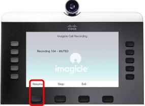
To stop recording, just hit the Stop button (it might be required to access again the Record service hitting the related key) or hang up.
