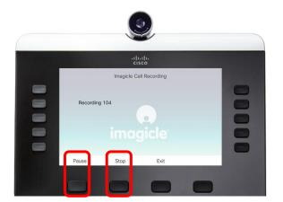
By hitting the Pause button, you can mute current recording. You can Resume/unmute the recording by hitting the related button, as in picture below.
