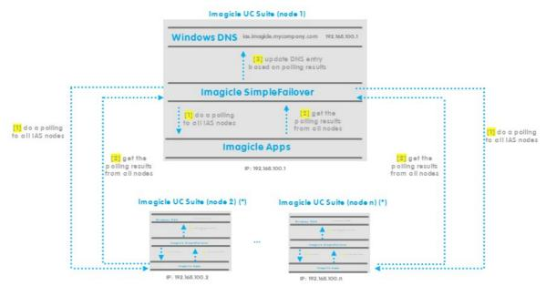
(\*) Imagide SimpleFailover must be installed on all Imagicle nodes and all instances do the same operations. For sake of clarity, this schema shows the interactions from a single Imagicle node's point of view www.imagide.com
