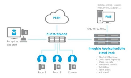
Imagicle Hotel Services communicates with the PMS through a permanent and bidirectional TCP link. The PMS vendor makes available an interface, which can be either hardware or software, usually installed at the Hotel. The purpose of the PMS interface is to let the PMS interface with external devices such as air conditioning, TV and PBXes. Imagicle Hotel Services is seen as a PBX.
