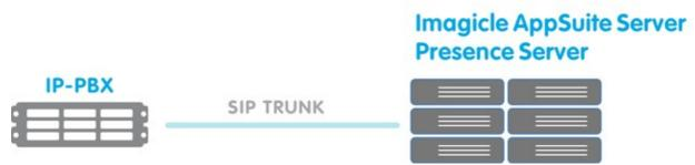
• With a Presence Server that supports SIP/Simple Presence interactions. Presence Server can be federated with an IP-PBX, this means that it will work as gateway for presence subscription requests coming from Presence Server and directed to IP-PBX, e.g. phone status requests
