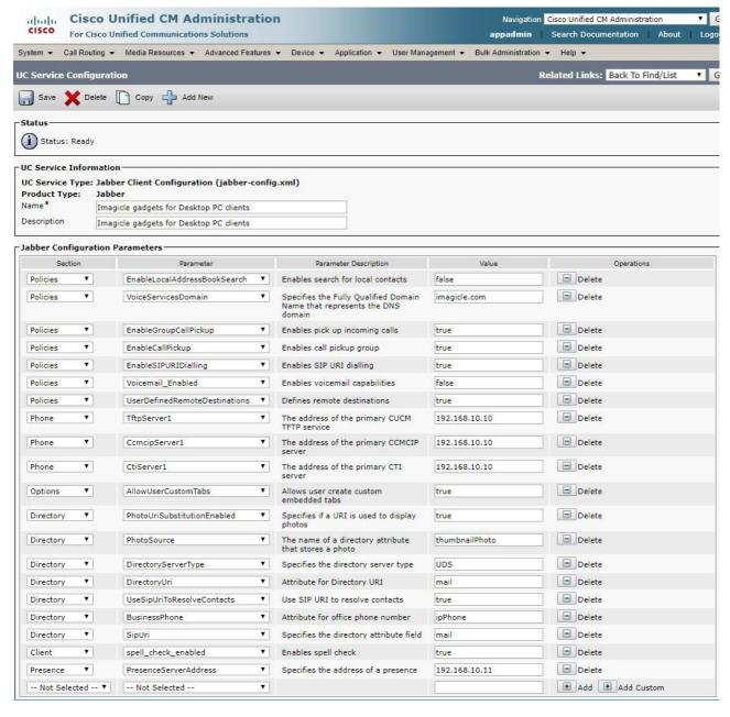
Then you can add a "Client" section for each Jabber Gadget to enable, following the sample below:
