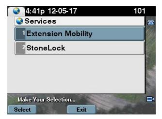
If the security PIN was never set, StoneLock will ask for a new PIN. In this case, enter the new PIN and confirm (see below).
